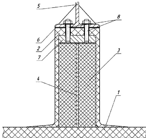
Fig. 3.44 Joint of a support element of an engine (equipment) to the seating closed box section with the use of studs and metal embedded parts:
