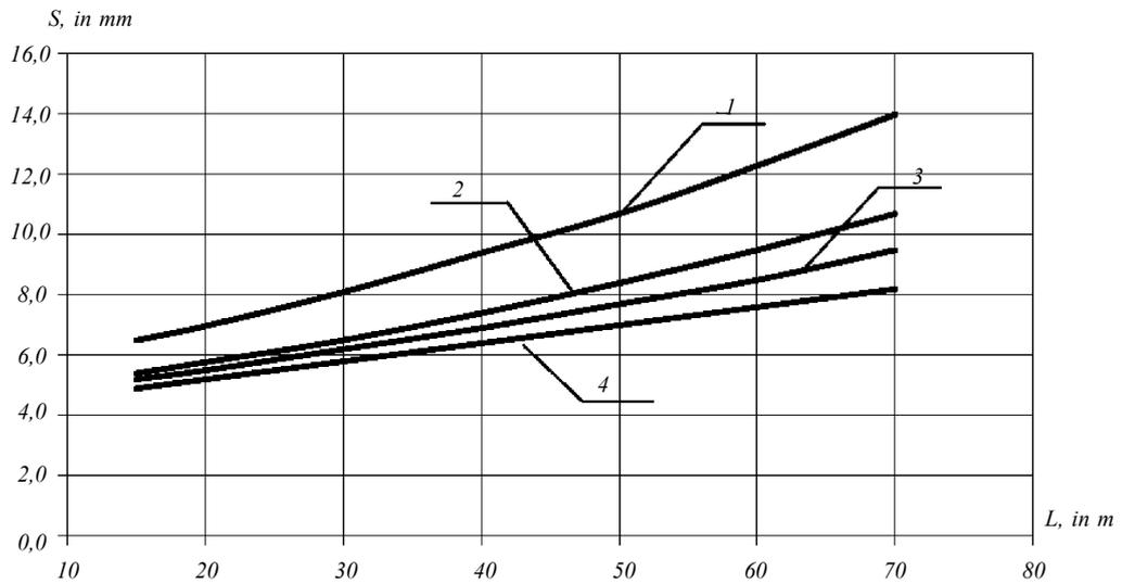
Fig. 3.7 Dependence of the minimum thickness of single-skin structures of the hull shell, deck and bulkhead plating manufactured of glass-reinforced plastic on the ship length
