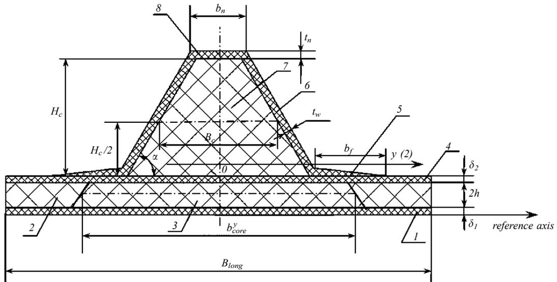
Fig. 1 Calculation method for the closed box (trapezoidal) member:
