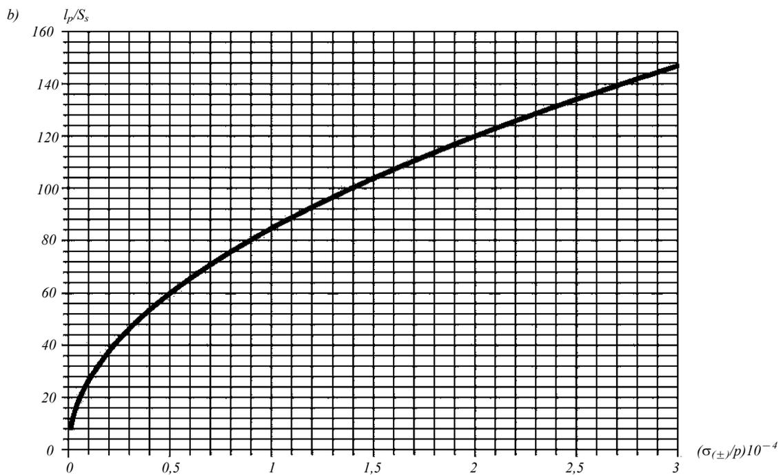
Fig. 3.5 Dependency diagrams of the maximum supporting contour length  $l_p$ , in m, of the laminate ratio to its thickness  $s_d$ , ( $s_s$ ), in m, and the ratio of laminate material properties  $E_p$ ,  $\sigma_{(\pm)}$ , in MPa, to design pressure  $p$ :
