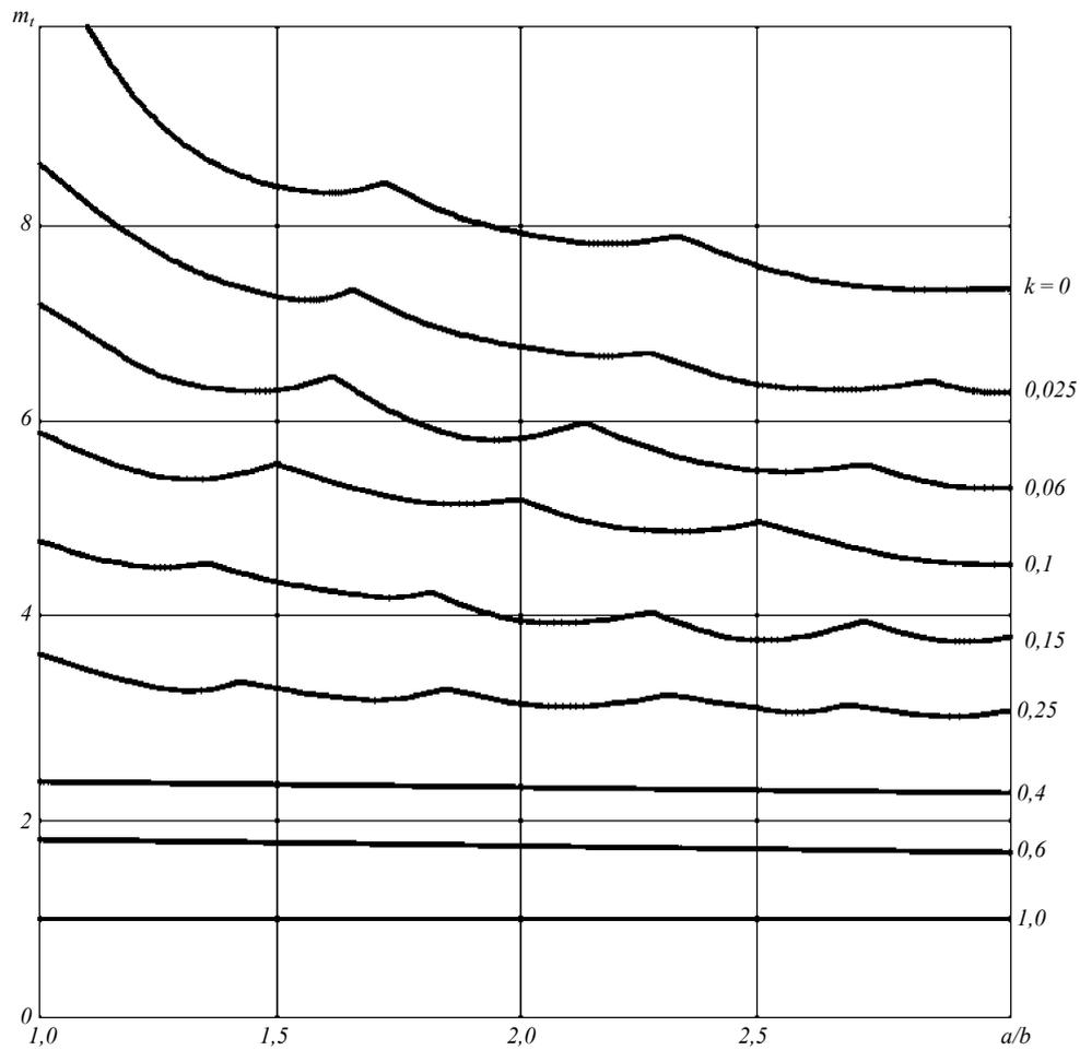
Fig. 33 Dependency diagram of factor  $m_t$  on ratio of plate sides  $a/b$  with all edges restrained
