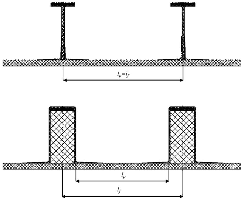
Fig. 3.6 Determination of the supporting contour length with framing members of different sections:
