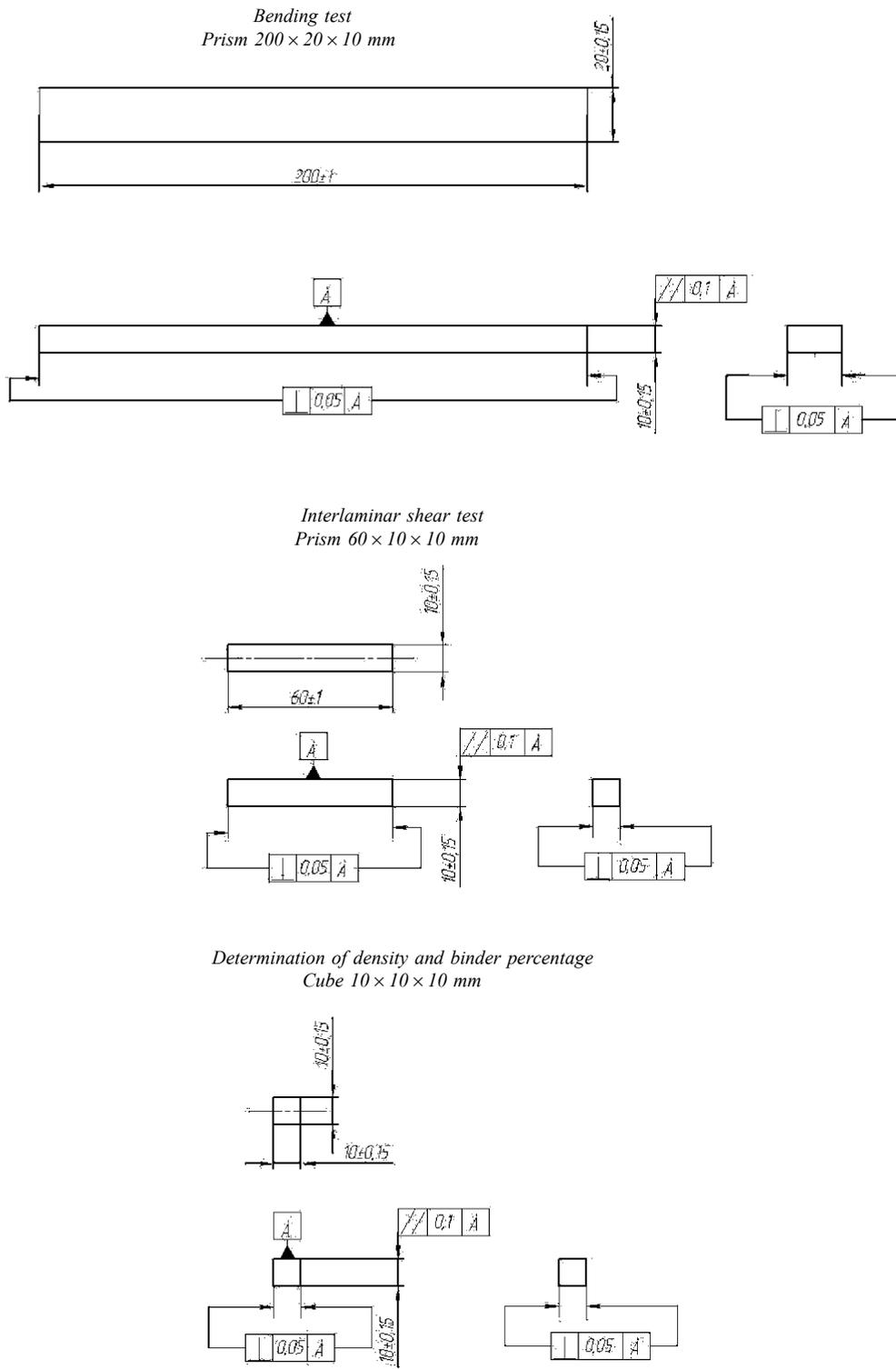
Fig. 2 FRP specimens for physical and mechanical tests in the initial state, cut out from laminates made of horizontal and vertical moulding (refer to Fig. 1)
