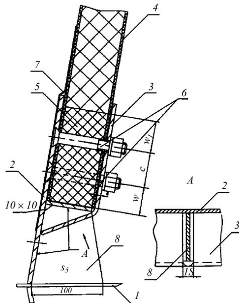
Fig. 3.52 Bonded and bolted joint of superstructure's side panels to the metal hull:
