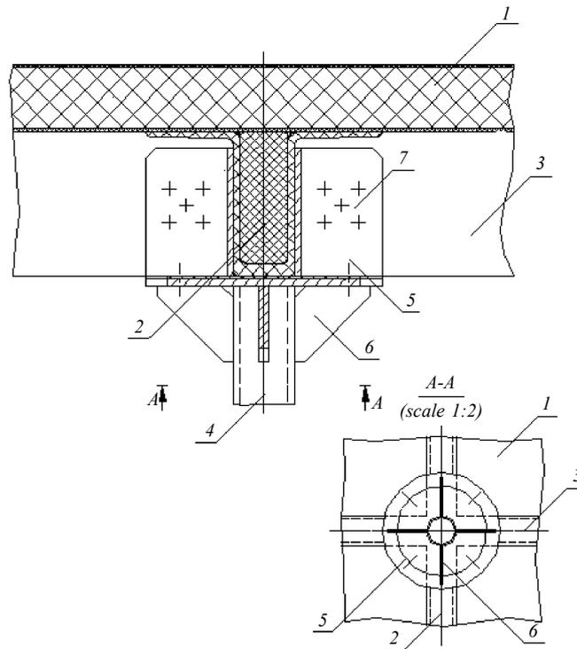
Fig. 3.50 Attachment of the upper end of an aluminum alloy pillar at the intersection of the superstructure beam and deck girder:
