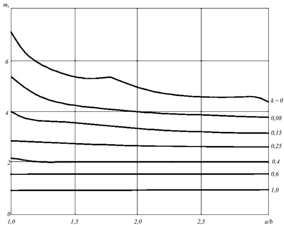
Fig. 35 Dependency diagram of factor  $m_t$  on ratio of plate sides  $a/b$ , with 1, 2 — hinge-supported; edges 3, 4 — restrained
