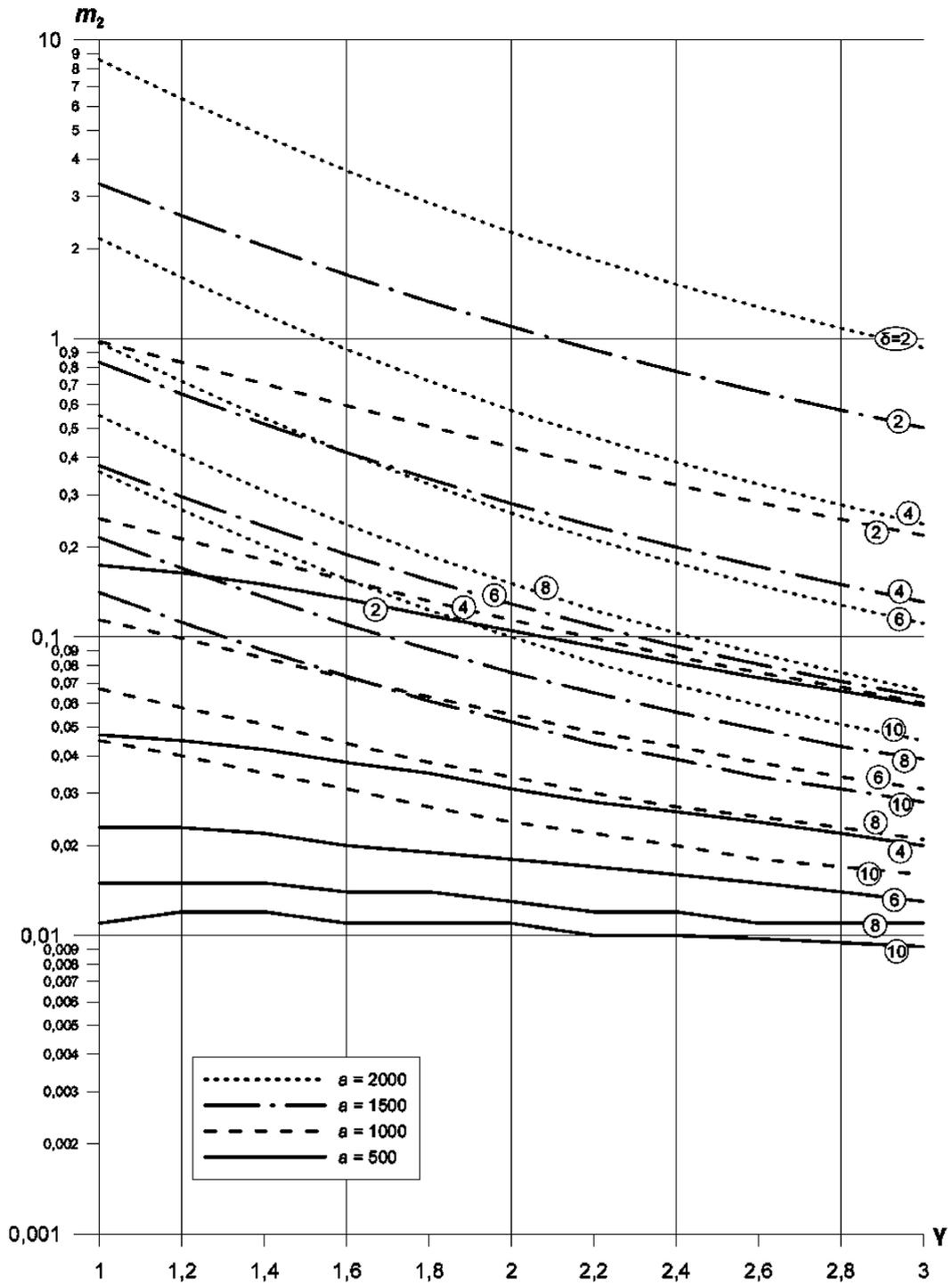
Values of thickness  $\delta$  of the sandwich plate load-bearing layer are shown in circles
