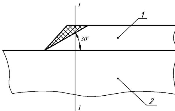
Fig. 5.2 Superstructure area (hatched) not considered in design cross-section ( $I - I$ ) when determine hull girder elements:
