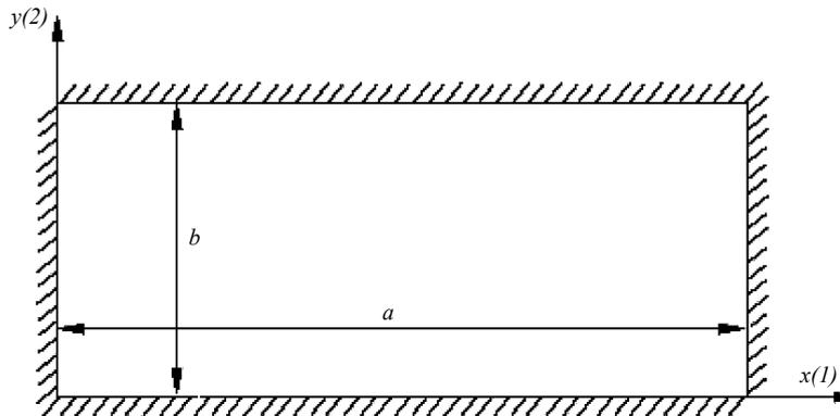
Fig. 3 Calculation method of single-skin plates
