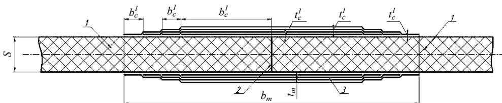
Fig. 3.31 Structural scheme of a moulded butt (seam) joint of single-skin members without edge preparation:
