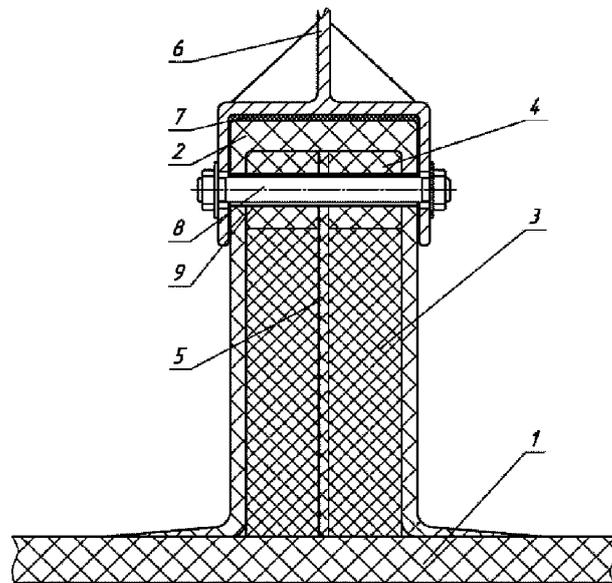
Fig. 3.43 Joint of a support element of an engine (equipment) to the seating closed box section with the use of bolts:
