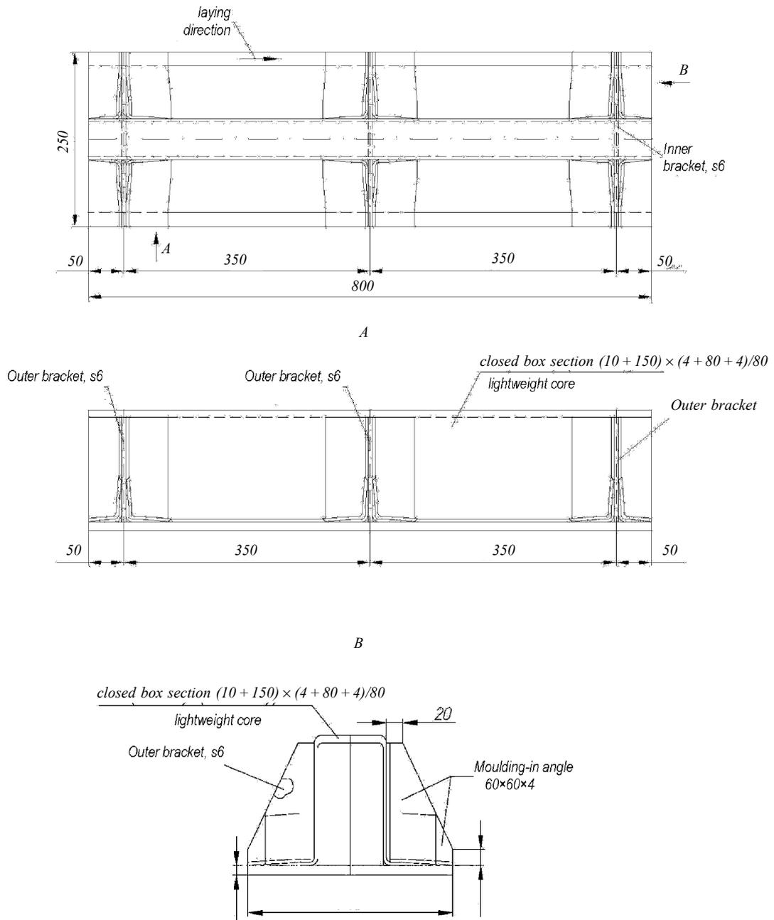
Fig. 4 General view of the closed box section framing members for short beam tests
