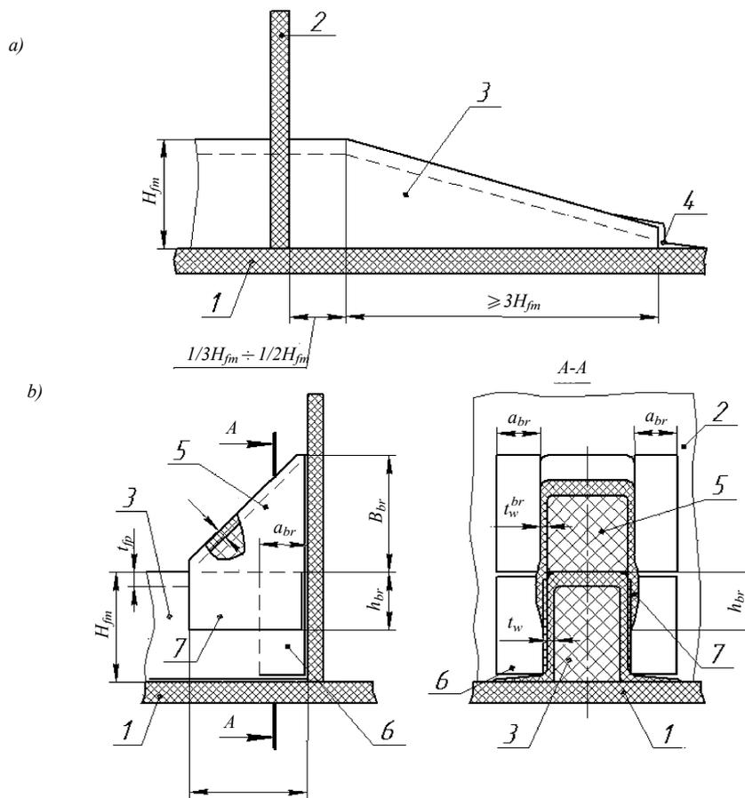
Fig. 3.19 Terminations of closed box section longitudinals:
