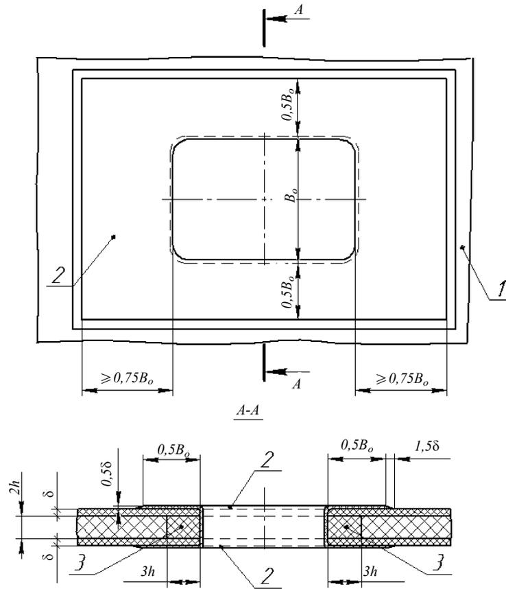
Fig. 3.30 Reinforcement of a rectangular opening in a sandwich structure:
