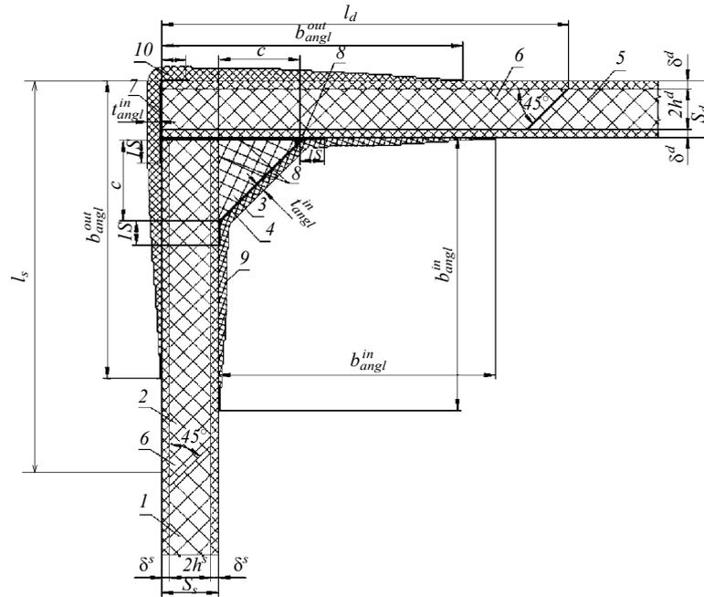
Fig. 3.38 Joint of the upper deck plating and side plating of sandwich construction (Type A):
