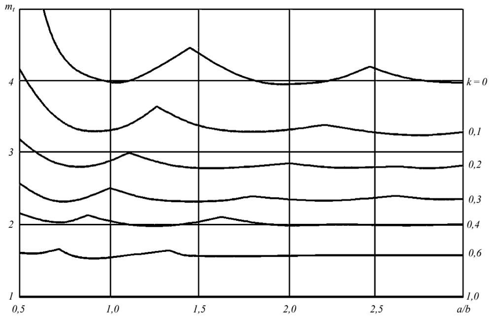
Fig. 32 Dependency diagram of factor  $m_t$  on ratio of plate sides  $a/b$ , with all edges hinge-supported
