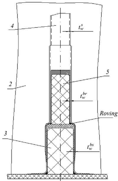
Fig. 3.24 Joint of the bulkhead stiffener and longitudinal (stringer, deck girder):
