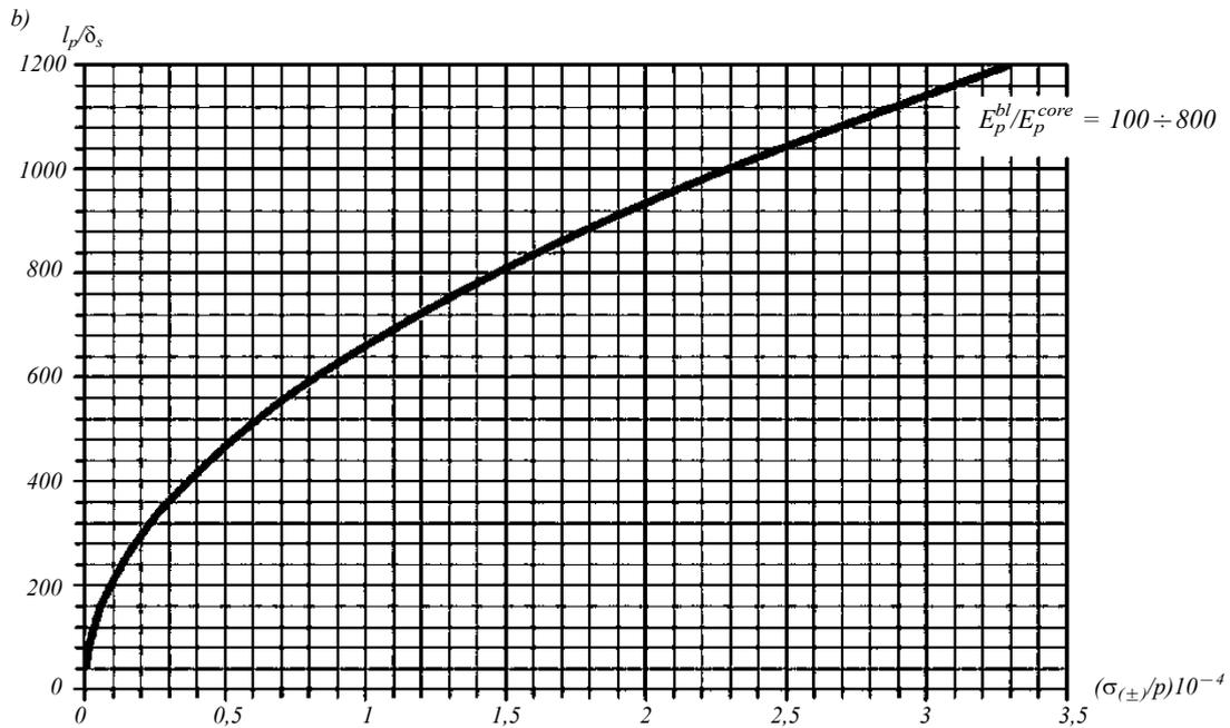
Fig. 3.9 Dependency diagrams of the maximum supporting contour length  $l_p$ , in m, of the sandwich laminate ratio to thickness of its load-bearing layers  $\delta_d$ , ( $\delta_s$ ), in m, and the ratio of laminate load-bearing layers' material properties  $E_p^{bl}$ ,  $\sigma_{(\pm)}^{bl}$  in MPa, to design pressure  $p$  (at  $2h=10\delta$ ):
