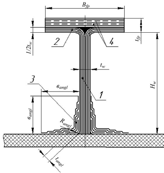
Fig. 3.16 Design of T-shaped section of framing members
