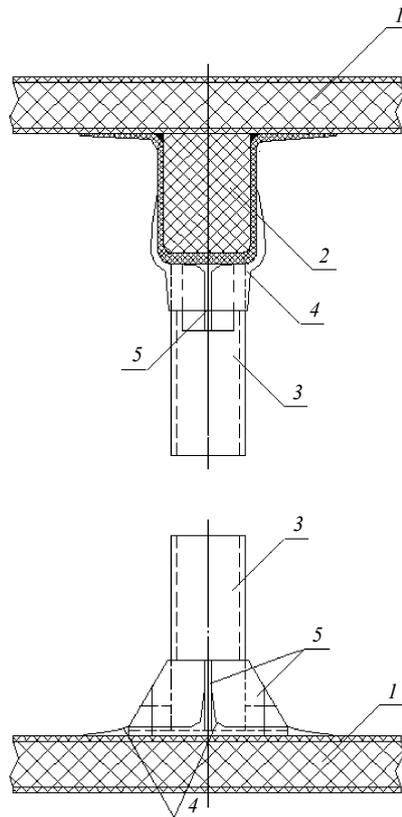
Fig. 3.51 Attachment of the FRP upper and lower ends to superstructure decks:
