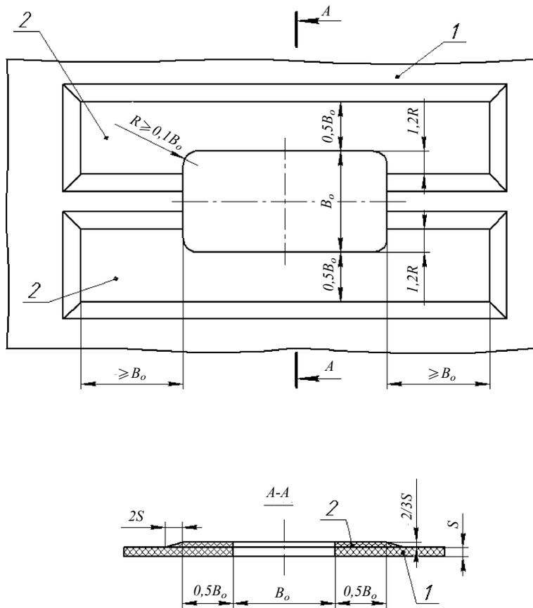
Fig. 3.29 Reinforcement of a rectangular opening in a single-skin structure:
