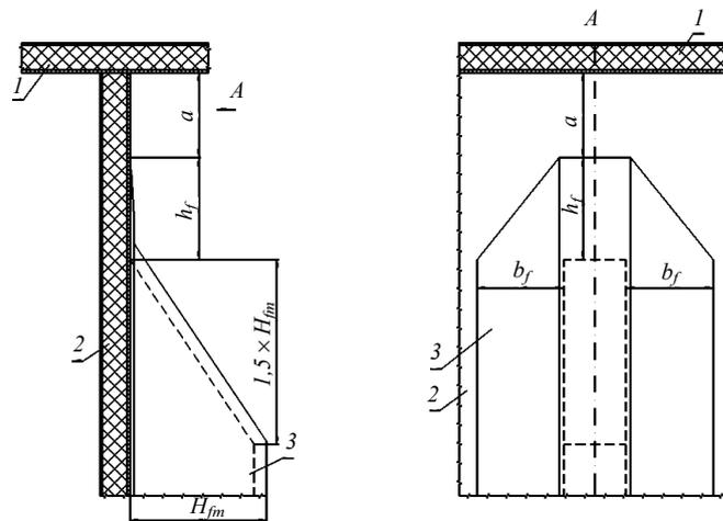
Fig. 3.26 Beveled termination of the bulkhead stiffener:
