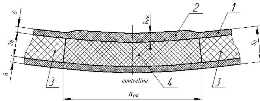
Fig. 3.11 Sandwich shell structure at the plate keel area
