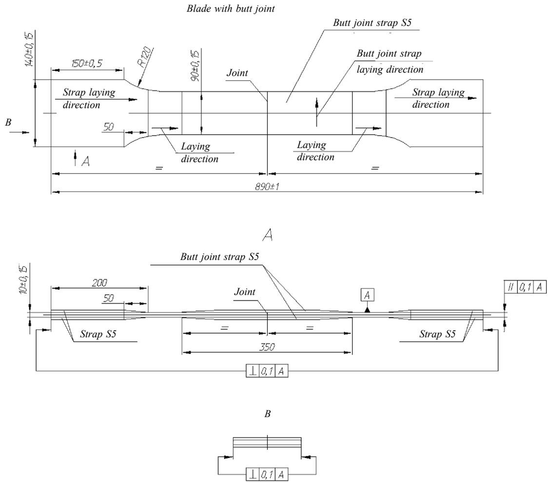
Fig. 5 Butt joint assembly for tensile testing
