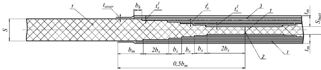
Fig. 3.32 Structural scheme of a moulded butt (seam) joint of single-skin members with double side stepped edge preparation:
