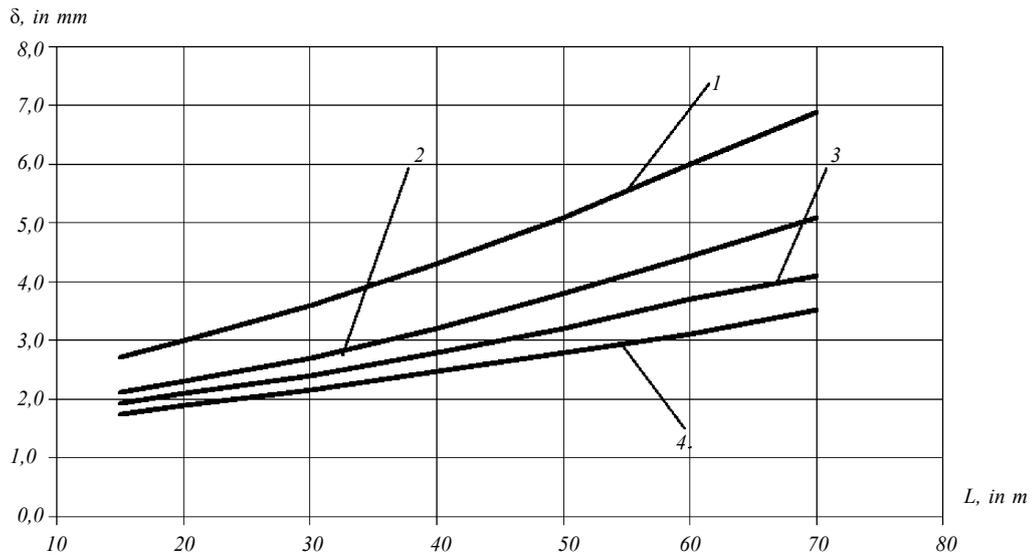
Fig. 3.10 Dependence of the minimum thickness of load-bearing layers of hull shell sandwich structures, deck and bulkhead plating on the ship length ( $L$  — length between perpendiculars):
