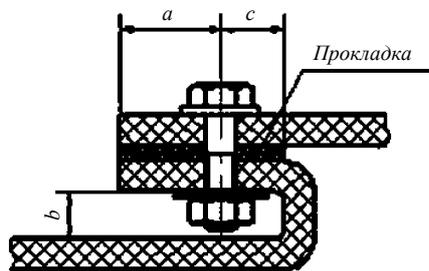
Fig. 3.47 Tank manhole assembly with the flanged shell
