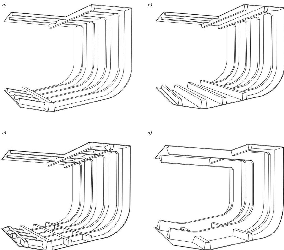
Fig. 3.2 Ship hull framing systems:
