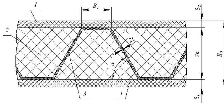
Fig. 3.12 Scheme of a deck sandwich laminate (bulkhead plating) with a corrugated element and foam plastic in a core
