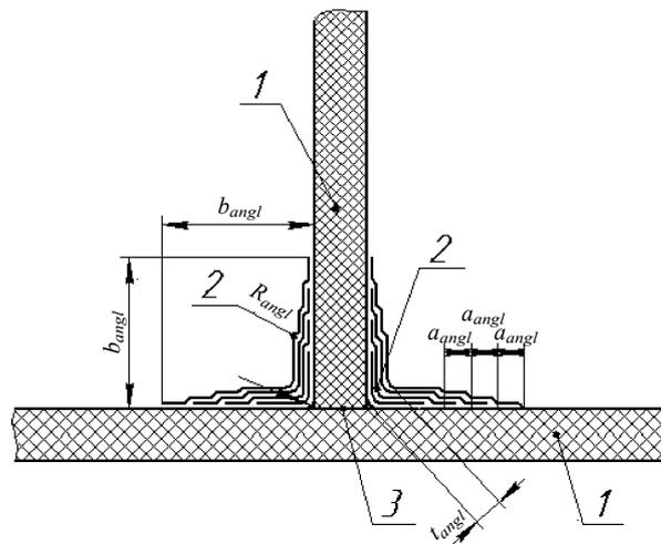
Fig. 3.34 Structural scheme of a moulded fillet joint:
