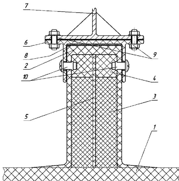
Fig. 3.45 Joint of a support element of an engine (equipment) to the seating closed box section with the use of a closed box flanged element made of FRP, bolts and rivet nuts:
