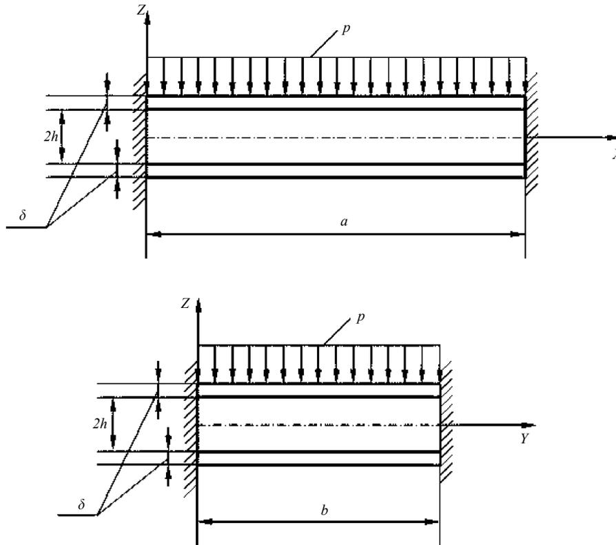
Fig. 25 Load type of the sandwich plate
