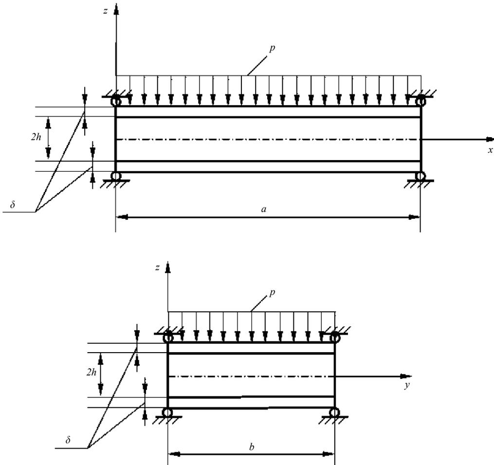
Fig. 9 Load type of the sandwich plate
