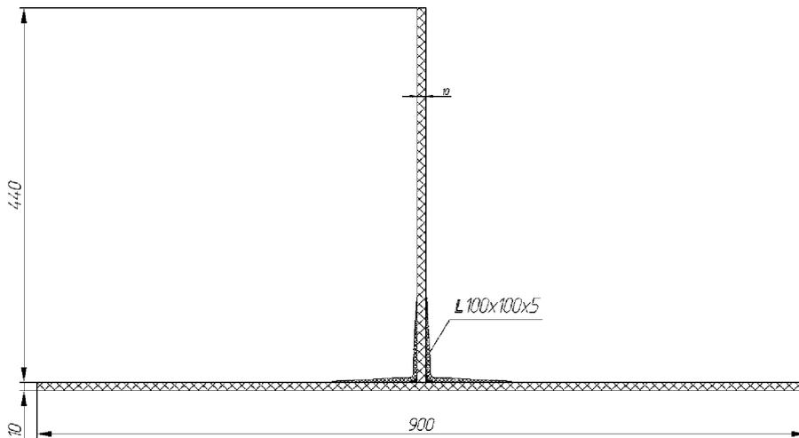
Fig. 6 T-joint assembly for uniform separation test
