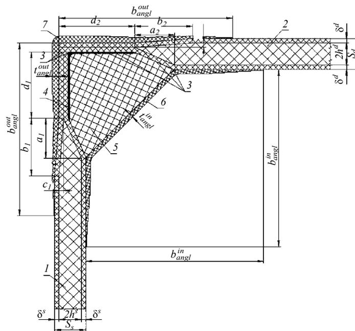
Fig. 3.39 Joint of the upper deck plating and side plating of sandwich construction (Type B):
