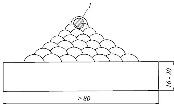
Fig. 4.8.4.4 Arrangements for cutting out specimens intended to determine  $\alpha$ -phase content by volumetric magnetic method:
