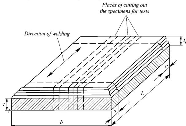
Fig. 4.8.3.5.2 Assembly imitating cladding deposit
