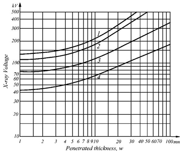
Fig. 3.2.4.5 The maximum X-ray device tube voltage values depending on the penetrated thickness of the controlled metal:
