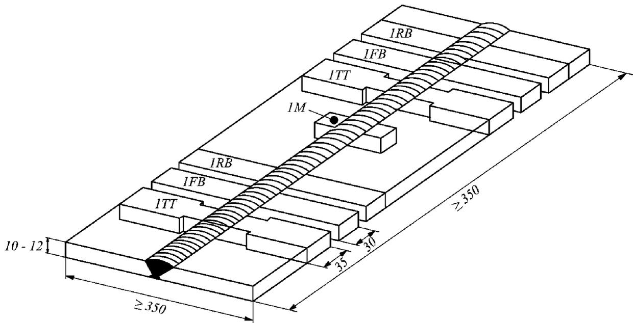
Fig. 4.9.3.1-1 Butt weld test assembly for welding in various welding positions:
