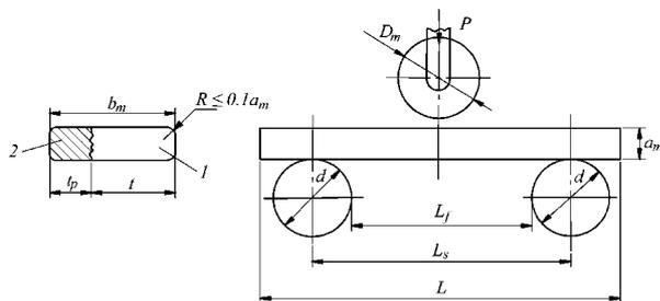
Fig. 4.8.4.2 Specimen with cladding deposit for side-bend testing
