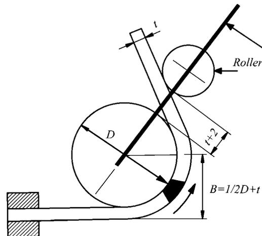
Fig. 4.9.3.6 Sketch of wrap around bend test
