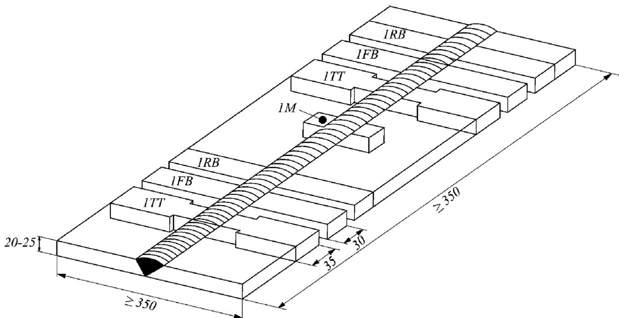
Fig. 4.9.3.1-2 Additional butt weld test assembly for welding in downhand position:
