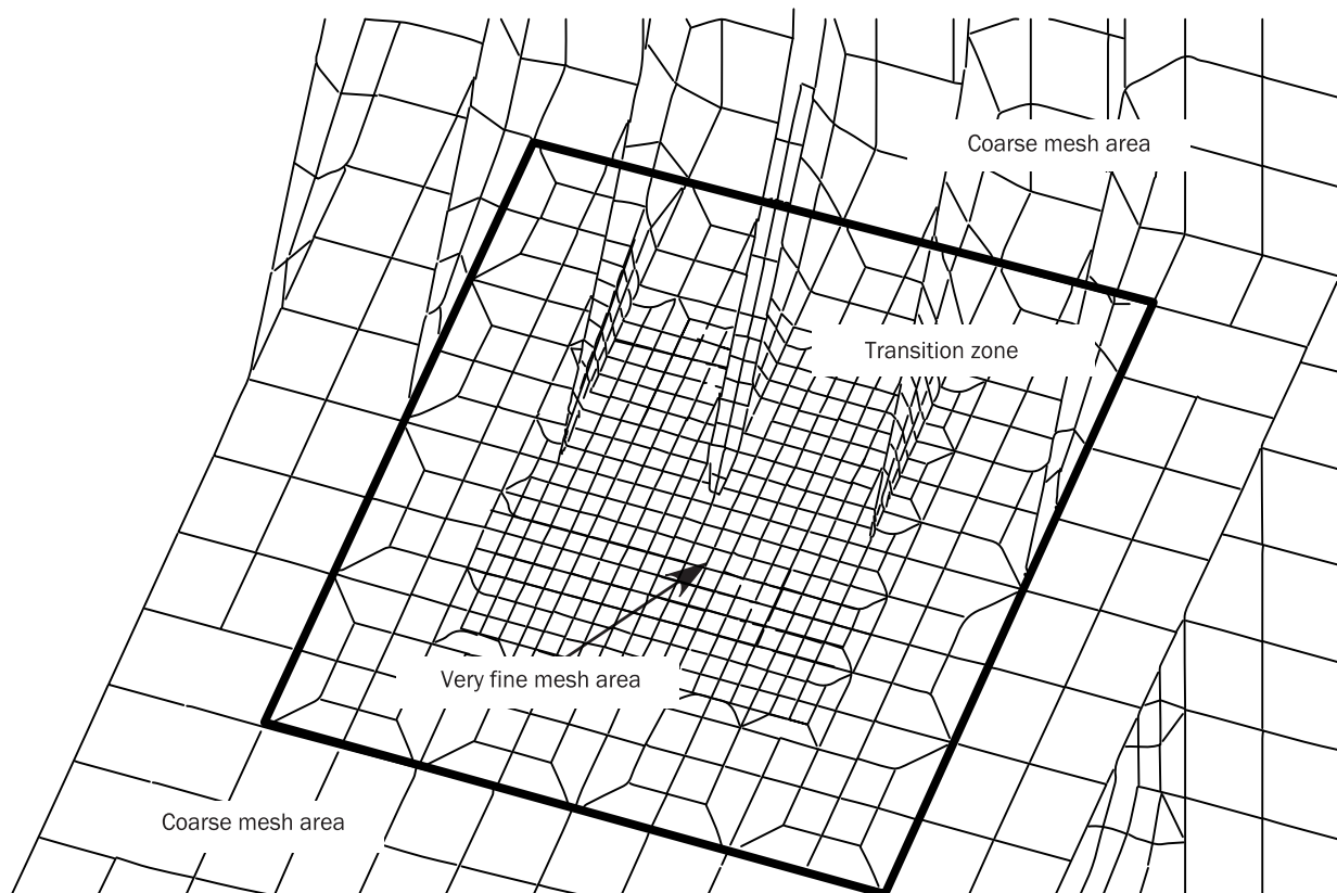
Figure 6 : Transition area between coarse and very fine mesh
