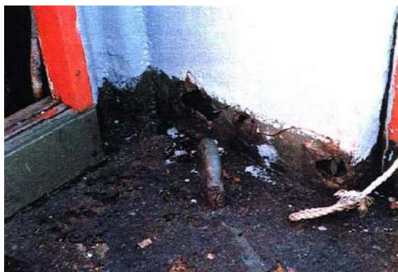
Photograph 1 Corroded accommodation house side structure
