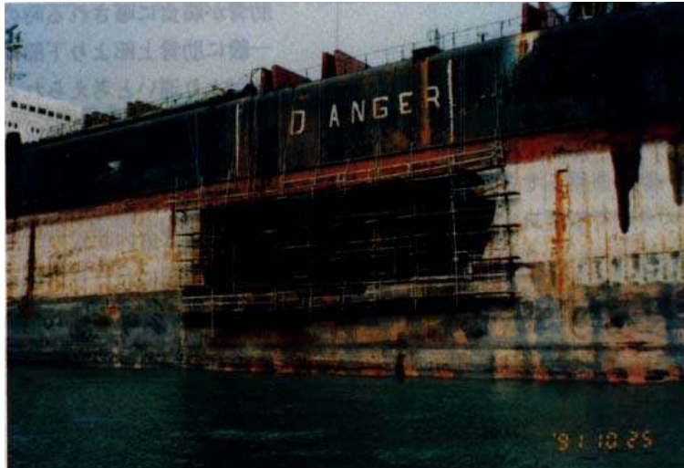
Photograph 2 Missing side shell structure (See Examples 4 and 5)
