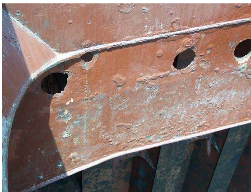
Photograph 2 Heavy corrosion of hatch coaming
