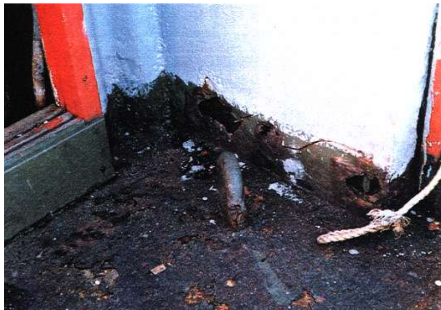
Photograph 1 Corroded accommodation house side structure
