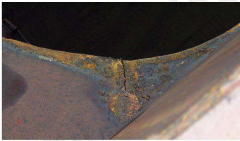
Photograph 3 Fractures at the hatch corner
