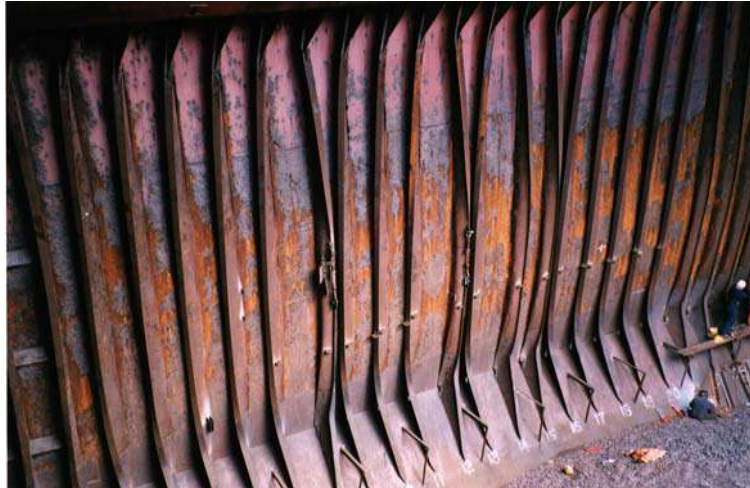
Photograph 1 Collapsed side shell frames (See Example 4)
