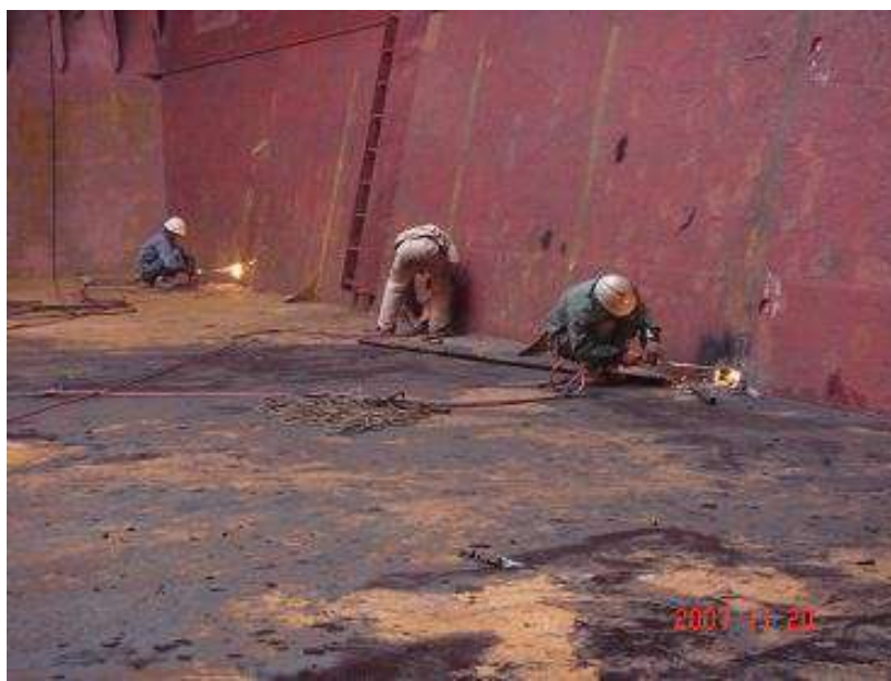
Photograph 1 Heavy corrosion affecting inner bottom plating
