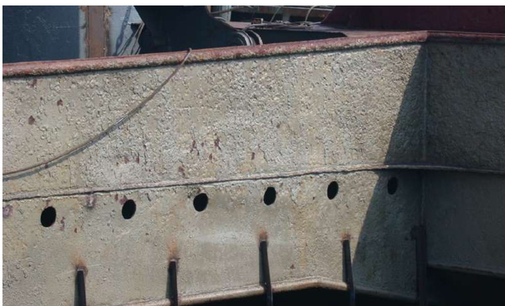
Photograph 1 Heavy corrosion of hatch coaming
