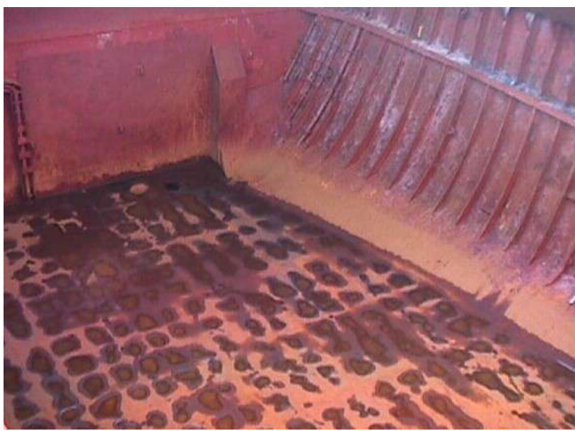
Photograph 2 Damaged inner bottom plating
