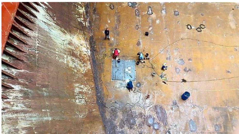
Photograph 3 Repairs of damaged inner bottom plating
