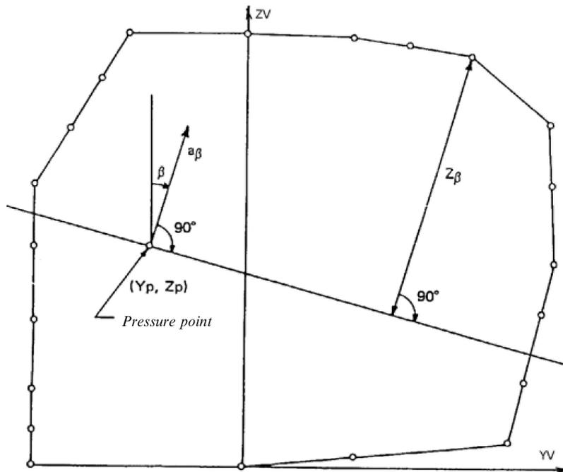
Fig. 28.1.2-2 Determination of internal pressure heads
