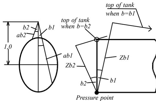
Fig. 23.1.4 Sketch for calculating a dynamic pressure differential
