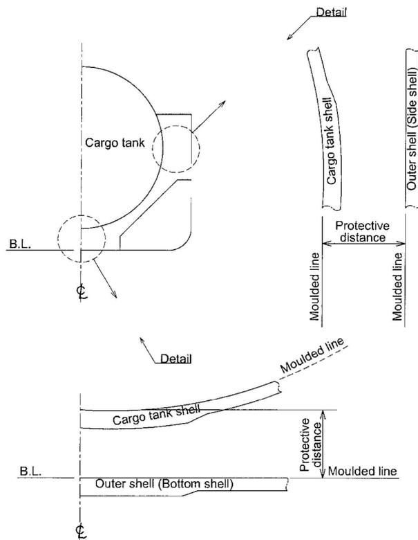
Fig. 2.5-5 Protective distance to pressure type tank
