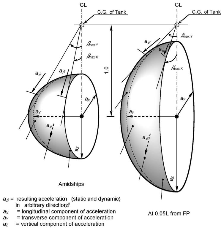
Fig. 28.1.2-1 Acceleration ellipsoid
