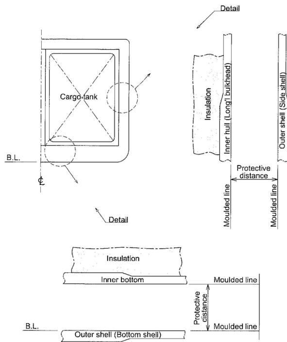
Fig. 2.5-2 Protective distance to semi-membrane tank
