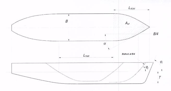
Fig. 2.1.1.4 Geometrical features of the ship for determination of the power delivered to the propeller shaft of ice ships
